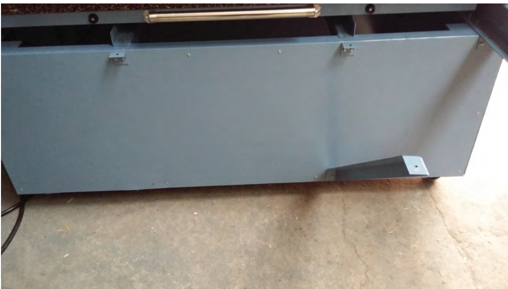
Picture No.4 - Fit the right hand side angle support
