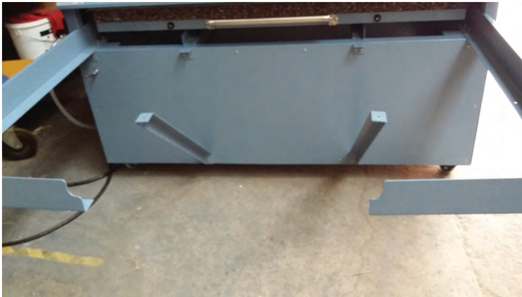
Picture No.5 - Fit the left hand side angle support
